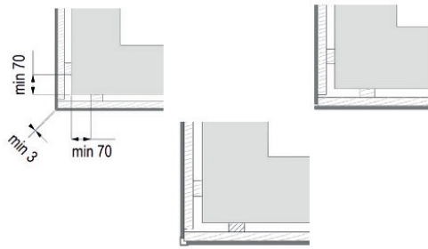
Facade corner details
